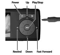
**Note:** To conserve battery power, the display dims after several seconds of button inactivity. Press the power button to restore the display.
